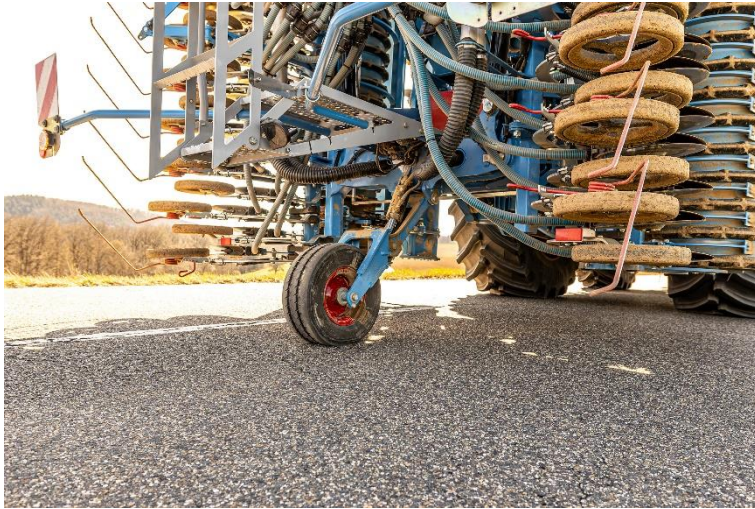
Image 3: The transport support wheel increases safety during road transport.
